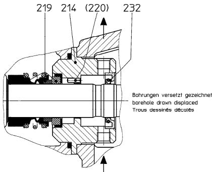
Permitted pressure at shaft seal  $p = -0,5$  bis 12 bar (16bar)
