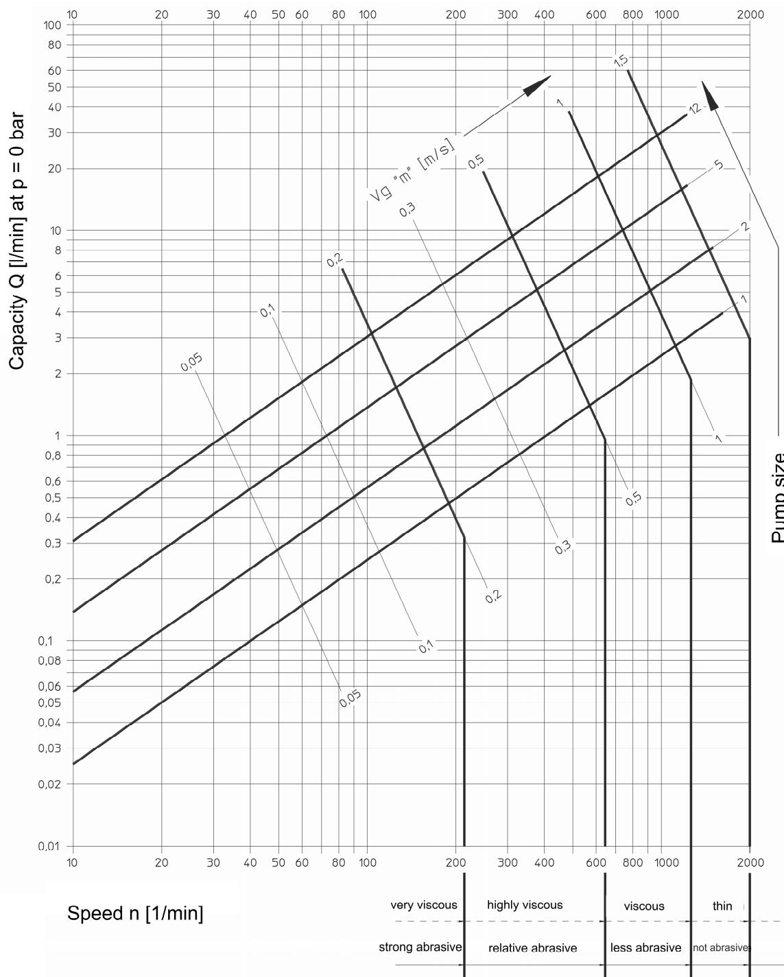
Sizes of series AEB DE. Refer to the separate individual characteristic curves for specifications on the performance range which are not covered by AEB DE series and for more detailed performance data.
